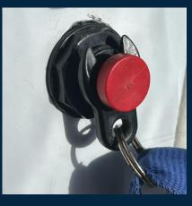
3. Twist key twice, the first will turn on battery, the second will start the engine (like a car)
